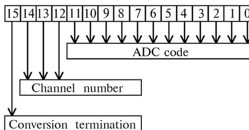
FIG. 2. The structure of the data and status register of the complex.
