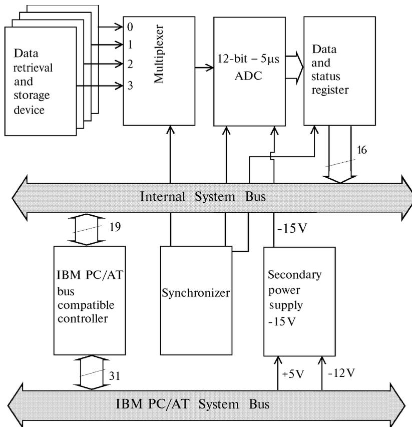
FIG. 1. Structural scheme of the hardware part of the complex.
