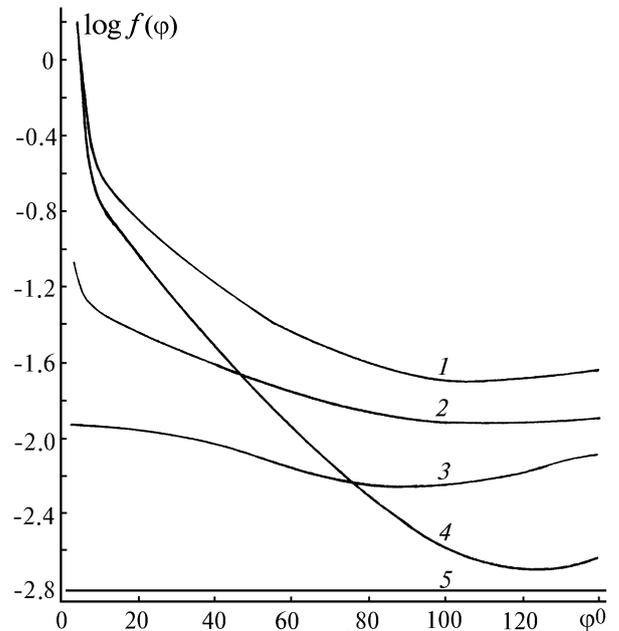
FIG. 1. Brightness phase function (1) and its components caused by multiple (2), single Rayleigh (3), and single aerosol (4) scattering, as well as the reflection of light from the underlying surface (5).
