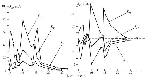
FIG. 1. An example of measured turbulent diffusion coefficients as a function of time.
