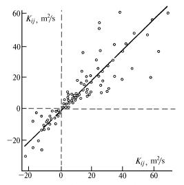
FIG. 2. The result of verification of the hypothesis (1):  $K_{ij}$  measured in accordance with Eq. (2) and calculated by Eqs. (1) and (3), m<sup>2</sup>/s. Solid line is the result of linear regression of the data.
