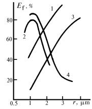
FIG 1. Efficiency of catching particles of different size in a human nasal cavity (1), in alveoles (2) and on third and fourth cascades of an impactor (curves 3 and 4, respectively).
