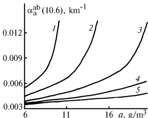
FIG. 2. Dependence of the submicron aerosol absorption coefficient in the 10.6 μm range on the absolute air humidity for  $m_d = 1.5$ ,  $\kappa_d = 0.7$  and five values of air temperature  $t = 12, 18, 24, 30, 36^\circ\text{C}$  (curves 1, 2, 3, 4, 5, respectively).
