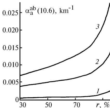
FIG. 1. Dependence of the submicron aerosol absorption coefficient in the  $10.6 \mu\text{m}$  range on the relative air humidity for three versions of  $\alpha_a^{\text{ab}}(10.6)$  calculations ( $m_d = 1.143$ ,  $\kappa_d = 0.07$  (1);  $m_d = 1.5$ ,  $\kappa_d = 0.7$  (2);  $m_d = 1.5$ ,  $\kappa_d = 1.5$  (3)).
