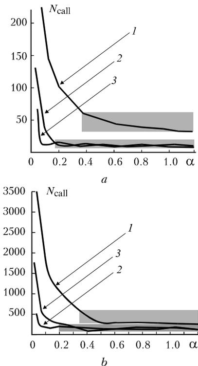
FIG. 3. Dependence of the speed of control on the parameter  $\alpha$  (the region of the optimal values of this parameter is hatched on the figure) for 1D (a) and 8D (b) objective functions. Curve 1 is for the trial variation method, curve 2 is for the modified trial variation method, and curve 3 is for the simplex method.
