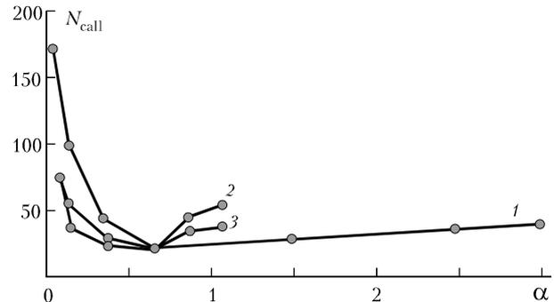
FIG. 6. Speed of control in a linear medium as a function of the parameter  $\alpha$ . Curve 1 is for the multidither algorithm, curve 2 is for the modified multidither algorithm, and curve 3 is for the simplex method.
