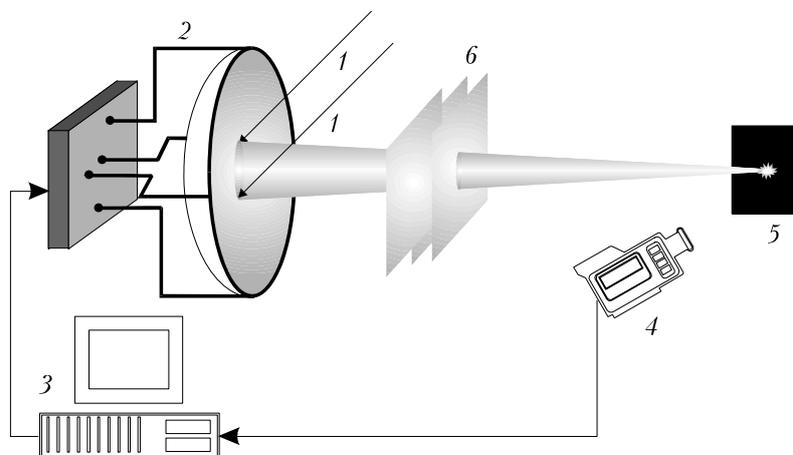
FIG. 1. Block diagram of the adaptive system: laser beam (1), adaptive corrector (2), generator of control signals (3), input system for data characterizing the field distribution (4), object of focusing (5), distributed thermal lens simulated by a set of screens (6).
