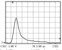
Fig. 6. The compressed ASE pulse waveform
