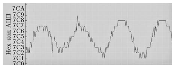
Fig. 5. The result of digitizing a small amplitude sinusoidal voltage.
