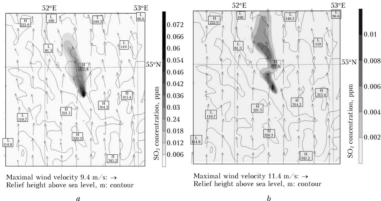
Fig. 2. SO<sub>2</sub> concentration at a height of 30 (a) and 70 m (b) 120 min later the emission beginning.
