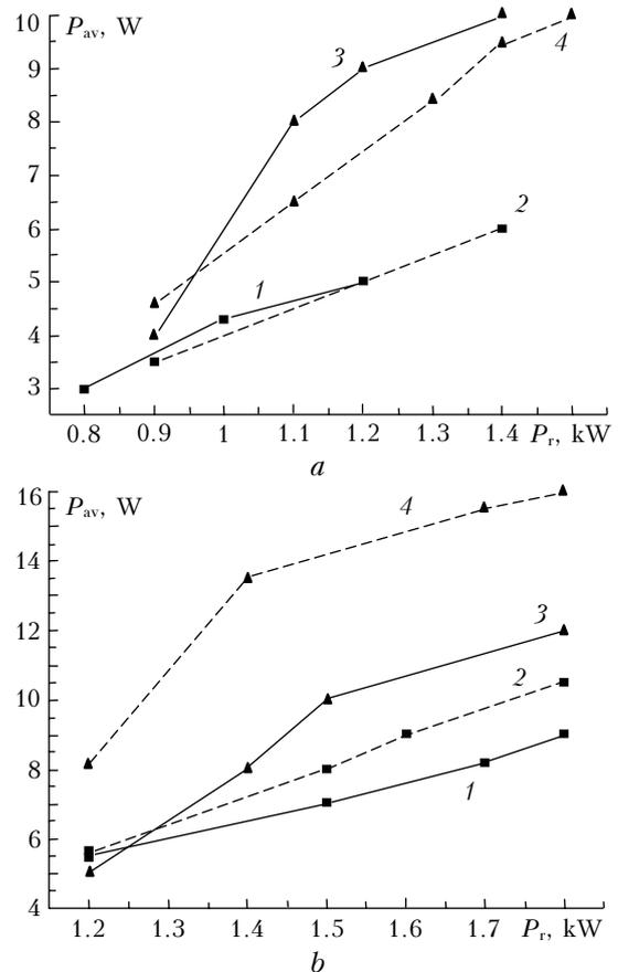
**Fig. 3.** Lasing power as a function of the high-voltage-rectifier-consumed power: GDT1 (a) and GDT2 (b). Curve 1 corresponds to the direct circuit, 2 – to the circuit with MPC, 3 – to the voltage doubling circuit, and 4 – to the voltage doubling circuit with MPC.
