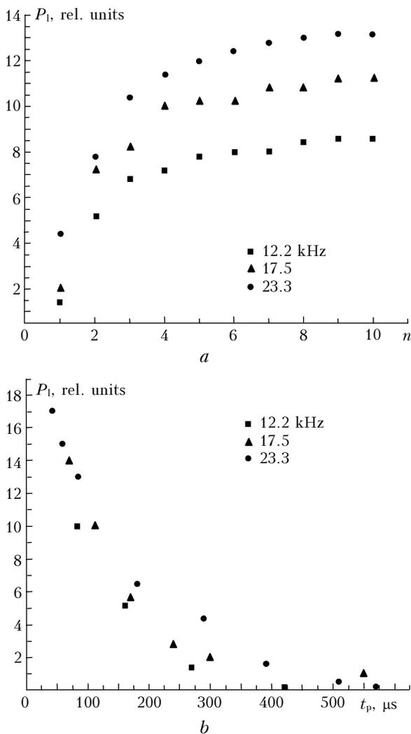
**Fig. 6.** Peak lasing power  $P_1$  as a function of pulse number in a train ( $a$ ) and the peak lasing power in the first pulse in a train  $P_{11}$  as a function of inter-pulse pause accumulating  $t_p$  ( $b$ ).
