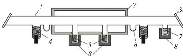
**Fig. 1.** Design of the active element of CuBr+Ne+HBr laser with low energy contribution in a discharge: GDT (1); heat chamber (2); windows (3); electrodes (4); containers with CuBr powder (5); traps (6); HBr generator (7); and heating elements (8).
