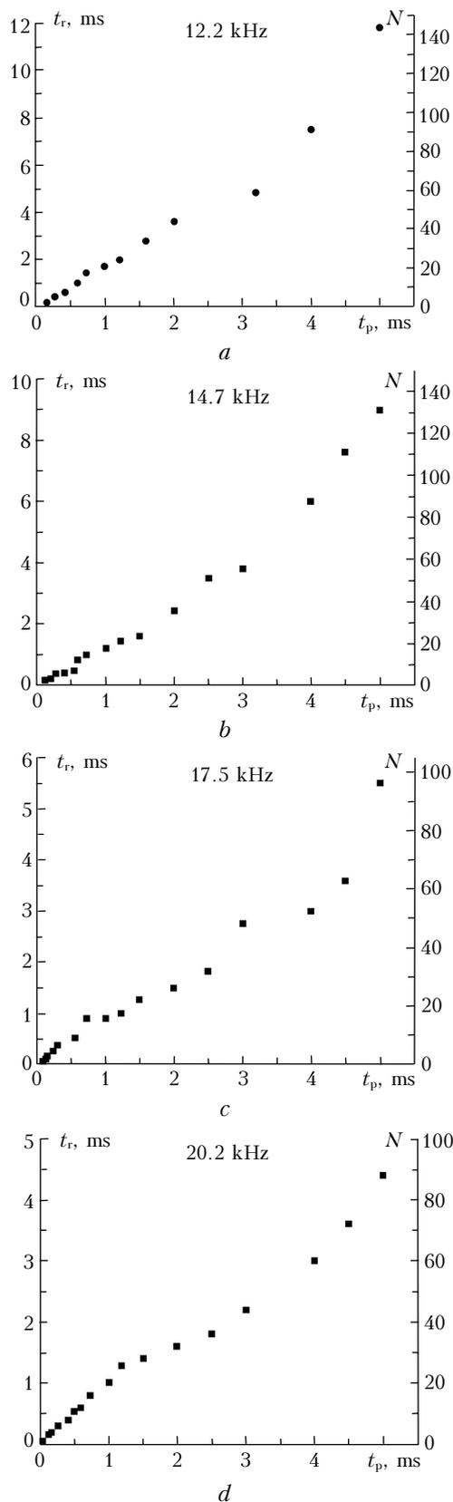
**Fig. 7.** The recovery time  $t_r$  ( $N$  pulses), required for attaining the maximum pulse power, as a function of inter-train period  $t_p$  at different pulse repetition frequencies in a train.
