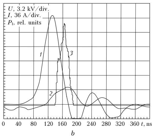
**Fig. 4.** Oscillograms of voltage (1), current (2), and lasing (3) for the voltage doubling circuit with MPC: GDT1 (a) and GDT2 (b).
