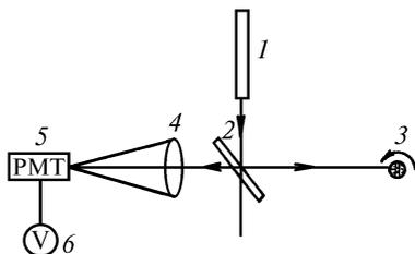
FIG. 1. Optical arrangement of the experimental setup.
