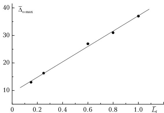
**Fig. 3.** The normalized mean width of the pulse frequency spectrum  $\bar{\Delta}_\omega$  depending on the light filament length  $\bar{L}_f = L_f/L_R$ : the calculated data are denoted by dots and the linear regression is presented by solid line.
