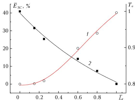
**Fig. 4.** Relative energy of supercontinuum  $\bar{E}_{\text{SC}}$  (1) and the coefficient of beam energy transfer  $T_e$  (2) as functions of the normalized length of light filament  $L_f$ ; the calculated data are denoted by dots; the spline-approximation is shown by solid lines.
