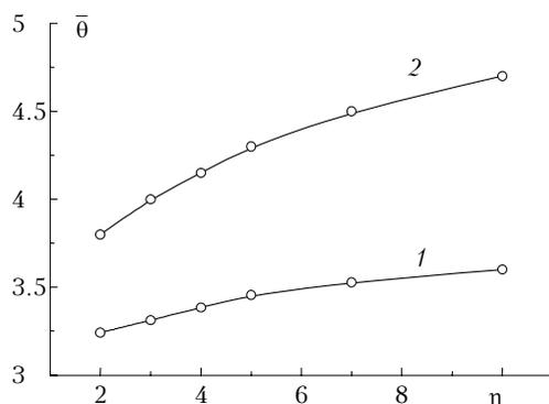
**Fig. 8.** The normalized angular beam divergence  $\bar{\theta}$  as a function of the initial power  $\eta$ . Dots present calculated data; solid lines are the spline-approximation;  $z = 1$  (curve 1) and  $z = 4$  (curve 2).
