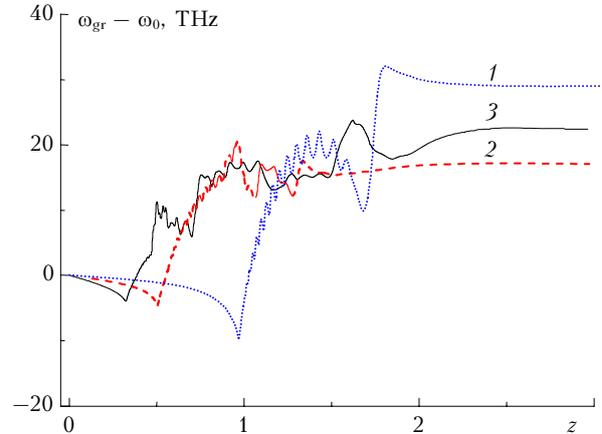
**Fig. 2.** The frequency of center of gravity of the pulse spectrum  $\omega_{gr}$  depending on the evolution variable for  $\eta = 2$  (1), 5 (2), and 10 (3).
