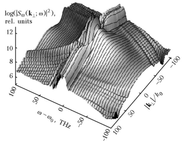
**Fig. 5.** The distribution of spectral intensity of a femtosecond pulse over the spatial and temporal frequencies at  $\eta = 5$  and  $z = 1.1$ .
