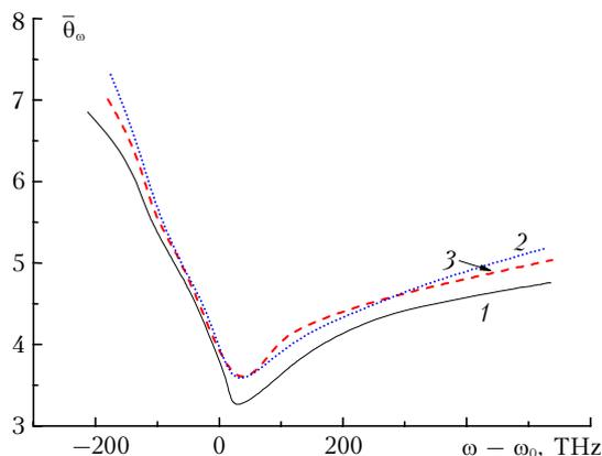
**Fig. 6.** Spectral dependence of normalized angular divergence of supercontinuum radiation  $\bar{\theta}_\omega = \theta_\omega / \theta_D$  at filamentation of a femtosecond pulse ( $\eta = 5$ ) in air at different distance  $z = 1.2$  (1); 1.5 (2); 2.0 (3).  $\theta_D$  is beam divergence due to diffraction.
