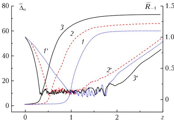
**Fig. 1.** Normalized mean width of the frequency range  $\bar{\Delta}_{\omega} = \Delta_{\omega}(z)/\Delta_{\omega}(0)$  (1–3) and the transverse beam radius  $\bar{R}_{-1} = R_{-1}/R_0$  (1'–3') at propagation in air of a femtosecond-duration radiation with the initial peak power  $\eta = 2$  (1), 5 (2), and 10 (3).
