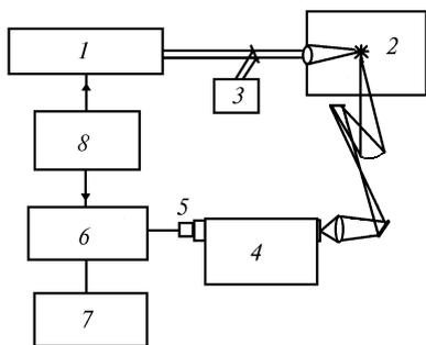
FIG. 1. The diagram of the experimental setup for spectrochemical analysis of the aerosols by breakdown plasma emissions spectra: CO<sub>2</sub> laser 1, hermetically sealed cell 2, IMO-2 power meter 3, MDR-6 monochromator 4, TV camera 5, graphics digitizer 6, computer 7, and block of synchronization 8.
