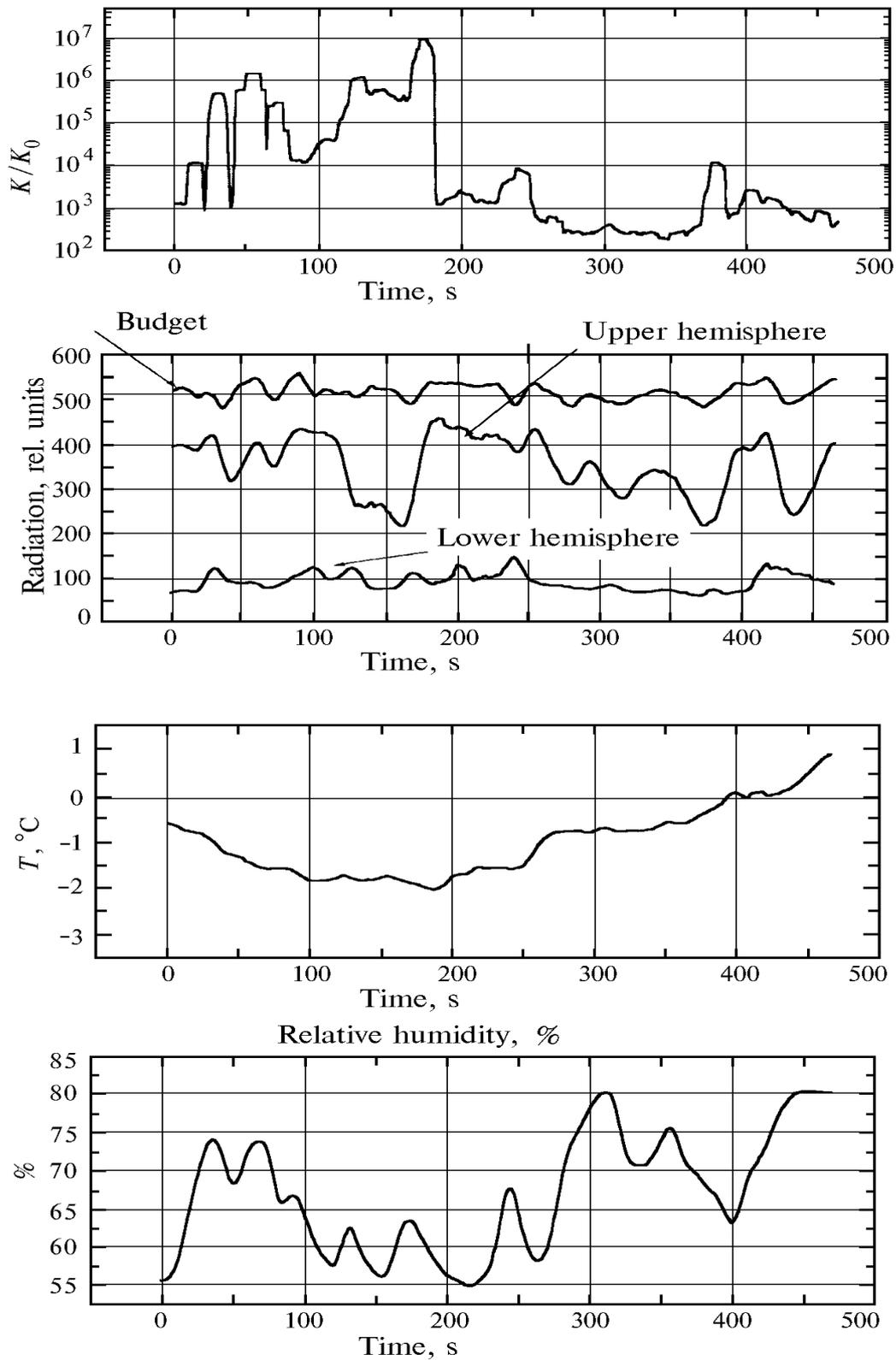
FIG. 3. Fragment of the data recorded by onboard computer when flying through the cumulus clouds in the vicinity of Tomsk. October 6, 1996.
