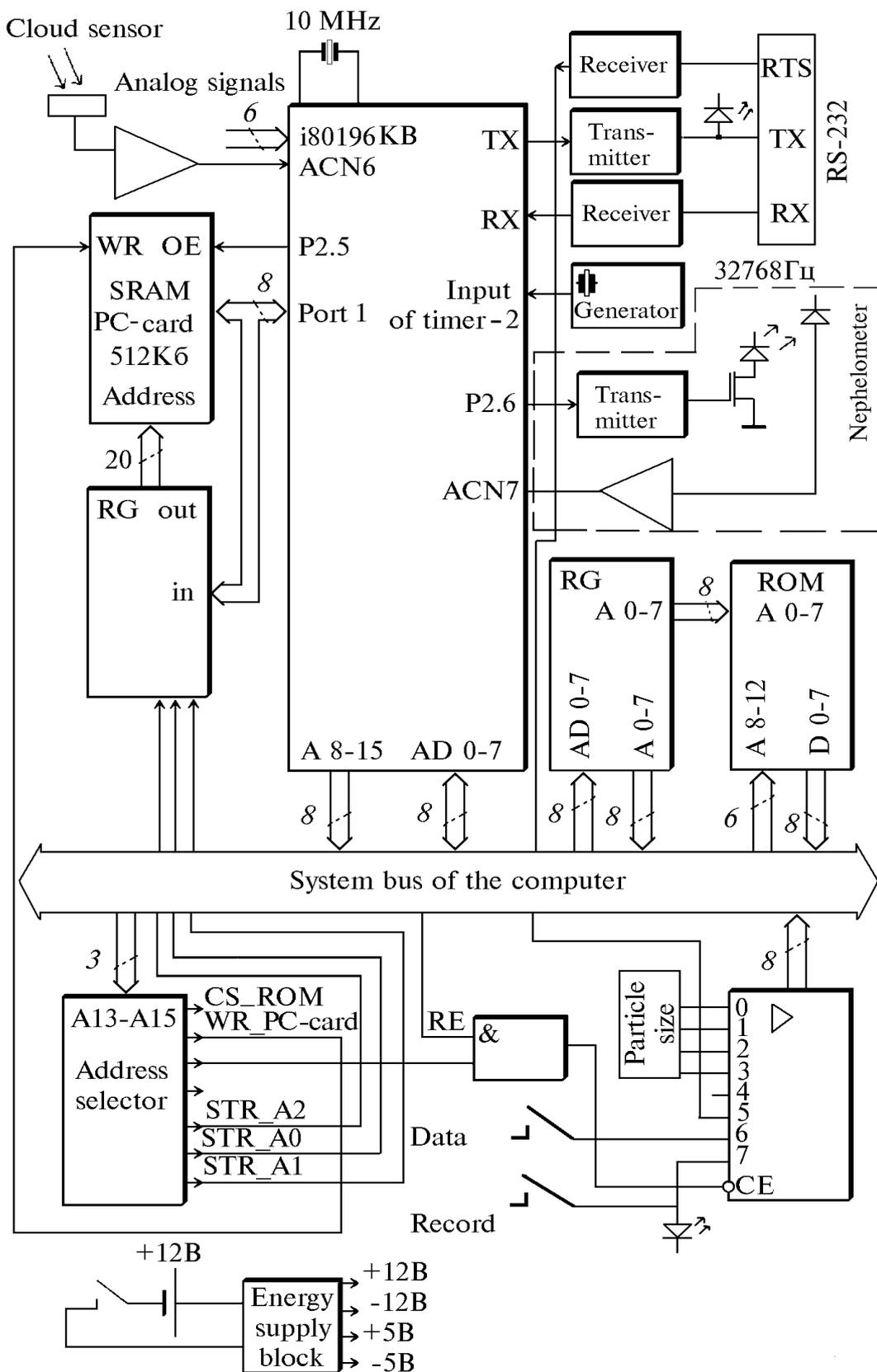
FIG. 2. Block-diagram of the system block of the complex.
