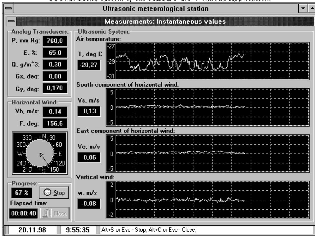
FIG. 3. METEO 2.0 Windows Application: the window for current measured data.
