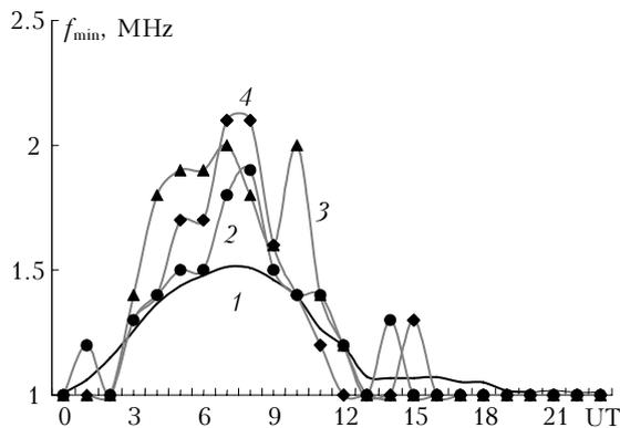
Fig. 4. The daily trend of  $f_{\min}$  (curve 1) averaged over January, February, and March, 1998, as compared to daily average trend during the days of the  $f_{\min}$  anomalous behavior: for January, 21 (2); for January, 22 (3); for January, 23 (4).
