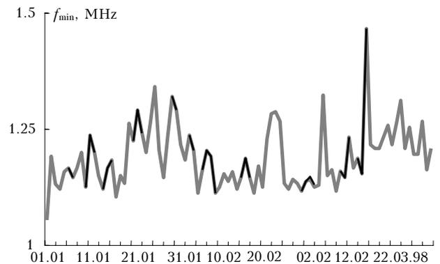
Fig. 6. Daily-mean trend of  $f_{\min}$  for January–March, 1998 from data of the Klyuchi station.
