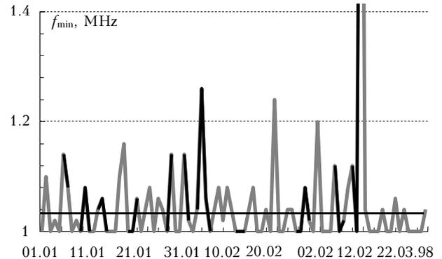
Fig. 5. Night-mean trend of  $f_{\min}$  for March and January, 1998.
