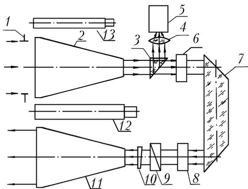
FIG. 2. Device for measuring the energy characteristics of the transceiver: 1) field stop ( $D = 75$  mm), 2) telescopic system, 3) prism, 4) condenser, 5) sensitive element of the energy meter, 6) constant optical attenuator, 7) rotating prism system, 8) variable optical attenuator, 9) wedge compensator for adjustment, 10) compensator for the velocity aberrations, 11) telescopic system, 12) collimator, and 13) sighting device.
