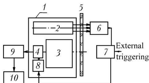
FIG. 3. Diagram of testing the lidar using the optical imitator of lidar signals: 1) transceiver, 2) laser transmitter, 3) receiving optical antenna, 4) photodetector block with interference light filter, 5) window of the orbital module, 6) photodetector, 7) electronic generator, 8) radiation source block, 9) SRLS, and 10) desk for testing SRLS.
