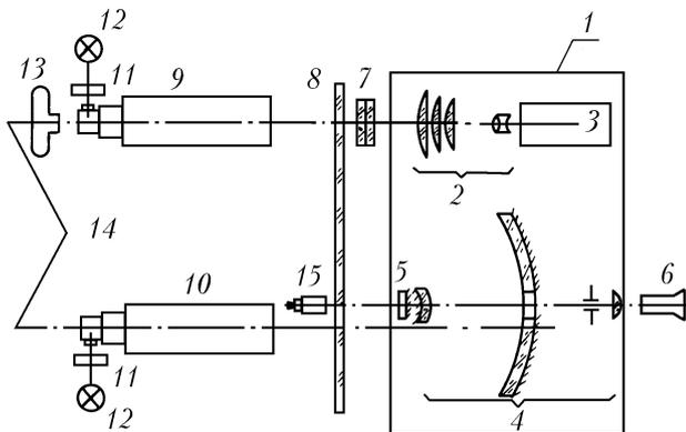
FIG. 1. Bench for testing the error in alignment of the transceiver of the lidar: 1) transceiver, 2) transmitting optical antenna, 3) laser, 4) receiving optical antenna, 5) alignment mirror, 6) dioptric tube, 7) neutral attenuating light filter; 8) plane-parallel plate, 9) and 10) collimators, 11) interference light filters, 12) light sources, 13) microphotographic attachment, 14) optical axes of optical benches, and 15) telescope.
