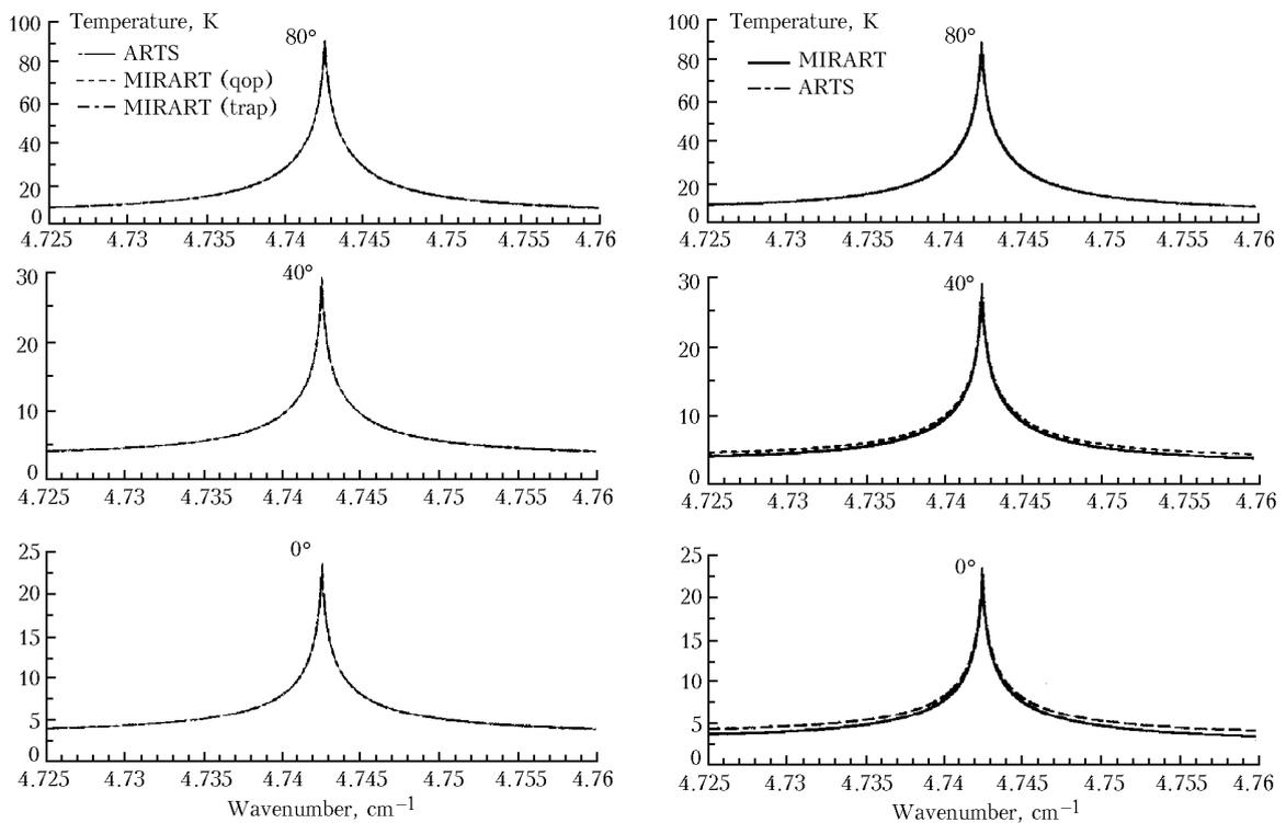
**Fig. 3.** IRTMW01 intercomparison: case 3 (left) and 4 (right) up-looking: ARTS line-by-line code (University of Bremen) vs. MIRART. (On the left "qop" and "trap" refers to "quadrature with overlapping parabolas" and "trapezoid quadrature", respectively, cf. subsection 3.4).  $\bar{T}_3$  and O<sub>2</sub>, perfect antenna (i.e., infinitesimal FoV), single side band receiver with Gaussian ILS function with half width 0.25 MHz.
