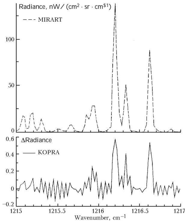
**Fig. 2.** AMIL2DA Forward model intercomparison (Exercise 20): KOPRA line-by-line code<sup>31</sup> and MIRART. Limb view with tangent altitude 40 km, apodized FTS instrument line shape, finite field-of-view. H<sub>2</sub>O, CO<sub>2</sub>, O<sub>3</sub>, N<sub>2</sub>O, and CH<sub>4</sub>; CKD-continuum.<sup>5</sup>
