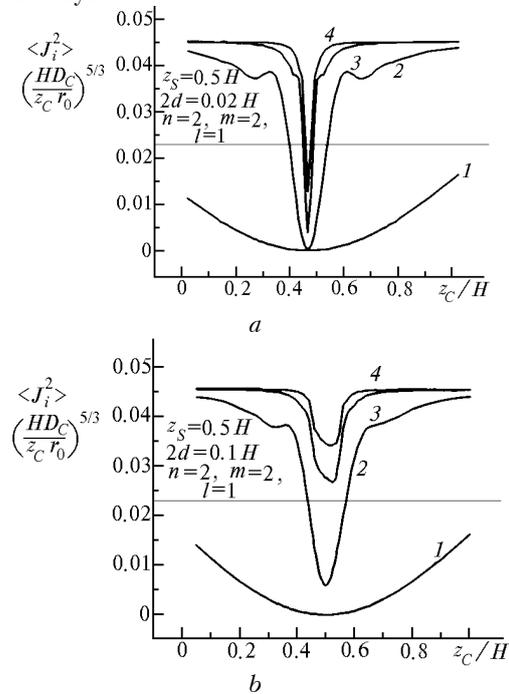
FIG. 2. Dependence of the residual error on the corrector position for different points on the object:  $\rho = 0.5R_c$  (1),  $\rho = 5R_c$  (2),  $\rho = 20R_c$  (3),  $\rho = 40R_c$  (4). The layer is in the middle of the path,  $z_S = 0.5H$  and has the thickness  $2d = 0.02H$  (a) and  $2d = 0.1H$  (b).
