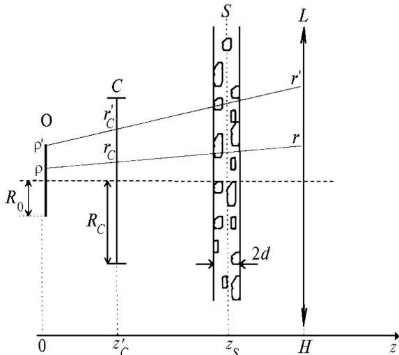
FIG. 1. Optical arrangement of an extended object imaging through the distorting layer of a turbulent medium. Here the object is designated as ( $O$ ), wave-front corrector ( $C$ ), layer ( $S$ ), and the receiving aperture ( $L$ ).
