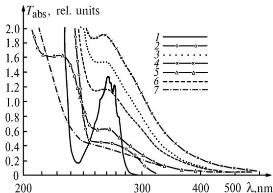
FIG. 1. The absorption spectra of oil products: gasoline (1), diesel fuel (2), Saratov oil (3), Georgian oil (4), Shaimskaya oil (5), and Libyan oil (6).
