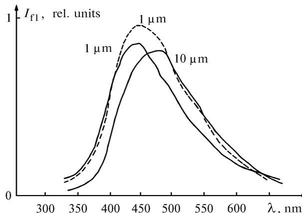
FIG. 3. The fluorescence spectra of the Libyan oil (solid curve, the cell thickness is 1 and 10  $\mu\text{m}$ ) and Saratov oil (dashed curve, the cell thickness is 1  $\mu\text{m}$ ).  $\lambda_{\text{ex}} = 308$  nm.
