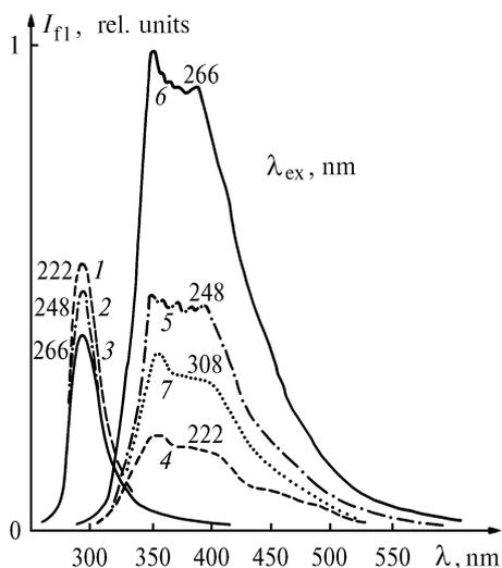
FIG. 2. The spectra of fluorescence of gasoline (curves 1–3, the cell thickness is 10  $\mu\text{m}$ ) and diesel fuel (curves 4–7, the cell thickness is 1  $\mu\text{m}$ ) at different wavelengths of excitation.
