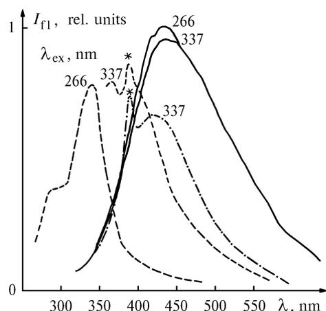
FIG. 4. The fluorescence spectra of Libyan oil. The line of the Raman scattering at  $\lambda_{\text{ex}} = 337$  nm is marked by asterisk.
