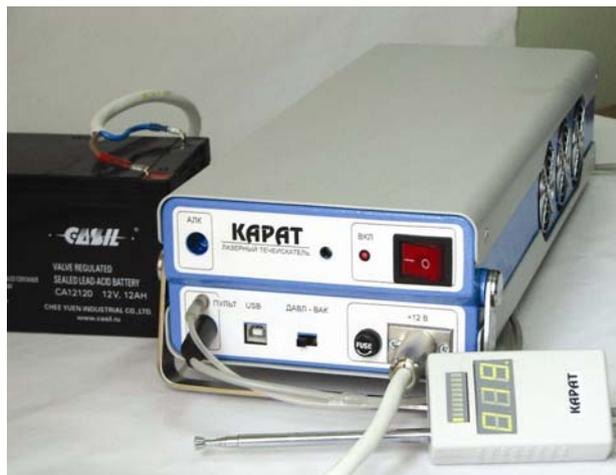
**Fig. 3.** Appearance of a “Karat” laser photoacoustic leak detector.
