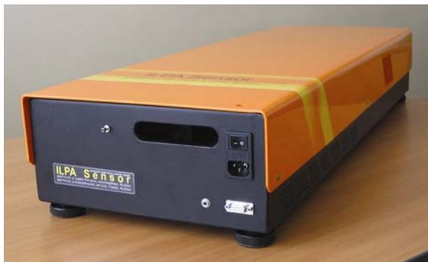
Fig. 5. Appearance of a laser gas analyzer with an intracavity PAD.
