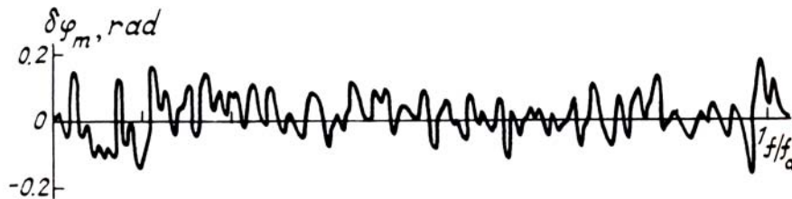
FIG. 1. Experimental plot of the error \delta\varphi_m in the Fourier spectrum of a point source obtained by Weigelt's method with 30 images as a function of the normalized spatial frequency f/f_d ( f_d is the diffraction frequency).
