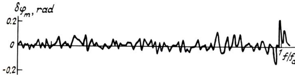
FIG. 2. Experimental plot of the error in estimating the phase \delta\varphi_m using the proposed iteration algorithm with 30 images as a function of the normalized spatial frequency f/f_d ( f_d is the diffraction frequency).
