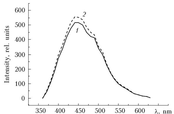
**Fig. 3.** Fluorescence spectra of the water solution of humic acid extracted from black soil, with allowance for IFE: the spectrum with a correction by the formula (5) (1); the spectrum with a correction by the Bouguer–Lambert–Beer law (2).
