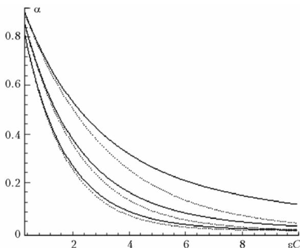
**Fig. 2.** The value  $\alpha$  as a function of the absorption coefficient  $\varepsilon C$  calculated by the formula (5) (solid lines) and by the Bouguer–Lambert–Beer law,  $\alpha = 10^{-\varepsilon C a}$  (dashed lines).  $R = 0.15$  cm, the curves (from bottom to top) correspond to  $a = R$ ;  $1.5R$ ;  $2R$ .
