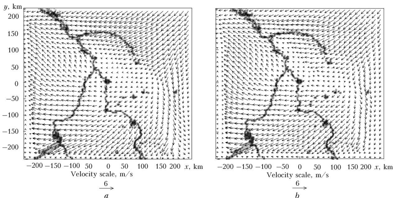
Fig. 2. Surface wind field for *D1* domain ( $450 \times 450$  km centered at  $85^\circ\text{E}$ ,  $56.5^\circ\text{N}$ ), calculated by the models MM5 (*a*) and WRF (*b*) for May 17, 2004, 8:00 p.m.
