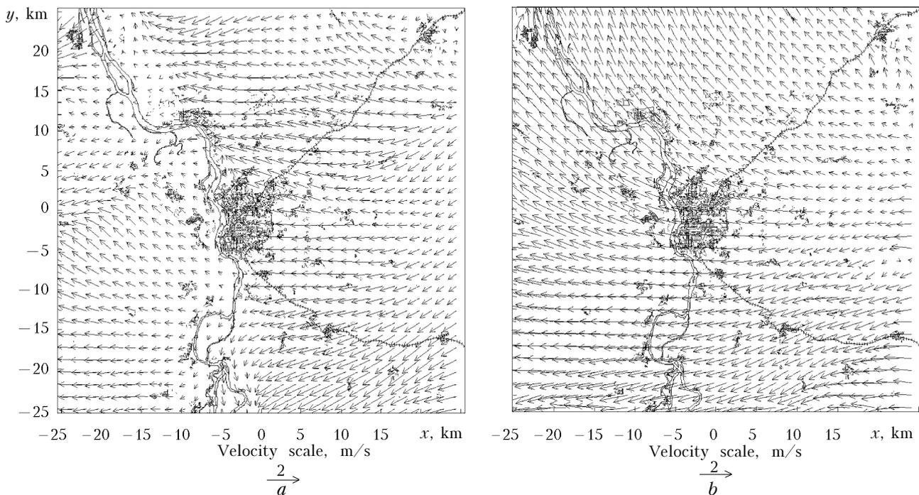
Fig. 3. Surface wind field for the *D3* domain ( $50 \times 50$  km, centered at  $85^\circ\text{E}$ ,  $56.5^\circ\text{N}$ ), calculated by MM5 (*a*) and WRF (*b*) for May 17, 2004, 8:00 p.m.
