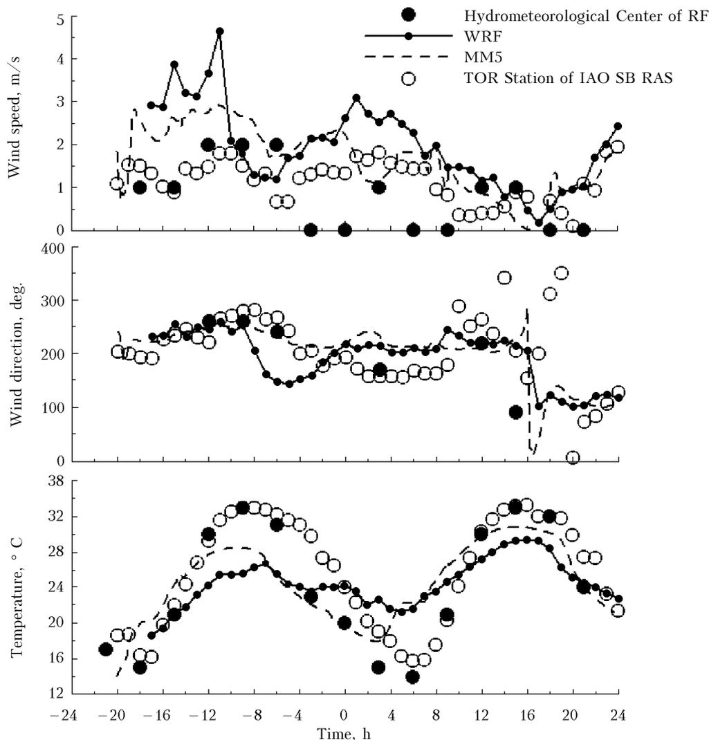
**Fig. 4.** The change in surface wind speed and direction, as well as surface temperature in Tomsk (85°E, 56.5°N) calculated by MM5 and WRF. Black circles refer to the observation data of the Russian Hydrometeorological Center, white circles are the data obtained at the TOR Station of the IAO SB RAS. Negative values refer to May 16, 2004, positive values refer to May 17, 2004.
