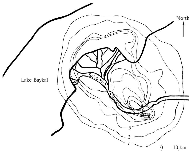
FIG. 1. Climatic distribution of the pollutants from Selenginsk pulp-and-paper mill (SPPM). The frequency of occurrence of the MM concentration exceeding MPC in December, shadowed rectangle designates Selenginsk City.
