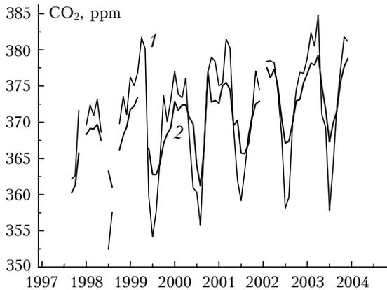
**Fig. 1.** Time behavior of the monthly mean CO<sub>2</sub> concentration in the atmospheric layers of 0.5 to 2 (1) and 3 to 7-km heights (2), obtained from monthly airborne measurements from onboard the An-30 Optik-E flying laboratory over forests of Southwestern Siberia.
