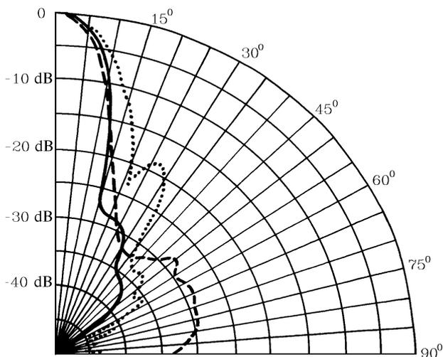
FIG. 1. The directional patterns of the ZVUK-1 sodar antenna at different stages of its manufacturing: the directional pattern of the paraboloid (dashed line), the directional pattern of the antenna with the shielding blend without a layer absorbing sound (dotted line), and the directional pattern of the finished antenna (solid line).
