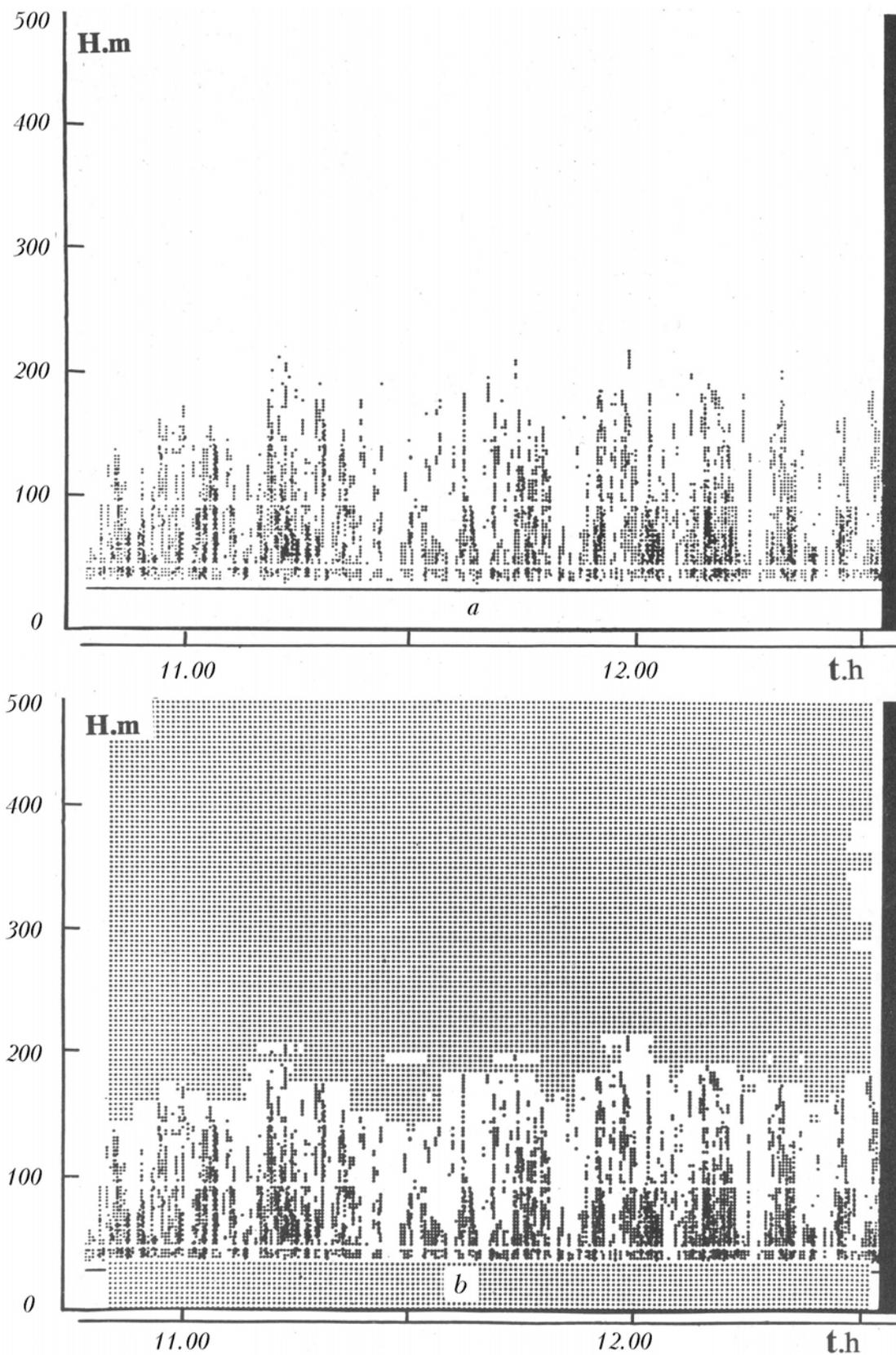
FIG. 3. Separation out of the echo-signal from the mixing layer on the facsimile recording: echo-signal recorded by the sodar (a) and mixing layer of the atmosphere detected by the sodar (nonshaded region) (b).
