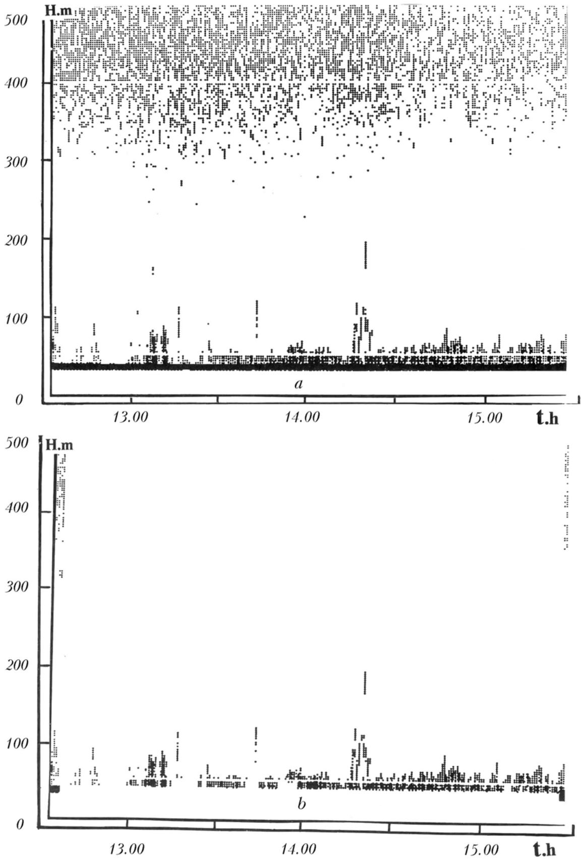
FIG. 2. The removal of noise from the facsimile recordings of the echo-signal: initial record (a), refined record (b).
