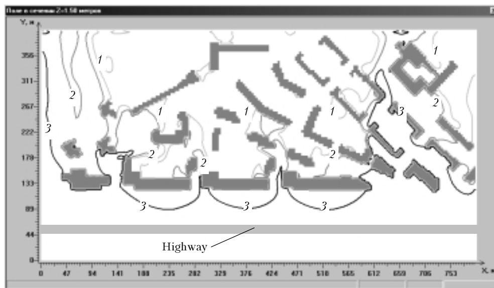
Fig. 1. Nitrogen dioxide concentration fields in the case of highway without protective shield. Isolines 1, 2, and 3 correspond to the concentration of 0.5, 1, and 2 MPC.
