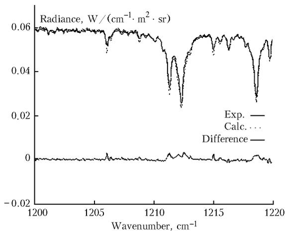
**Fig. 11.** Fitting of the IMG spectrum and spectrum simulated based on the retrieved water vapor concentration profile (see Fig. 9).
