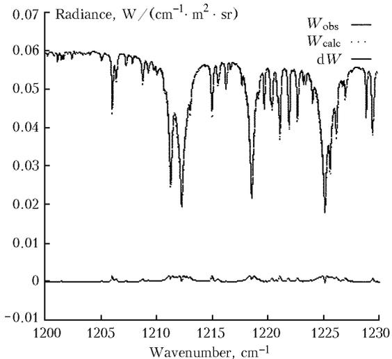
**Fig. 5.** Fitting of the initial model spectrum and spectrum simulated based on the retrieved profile of water vapor concentration (see Fig. 3).
