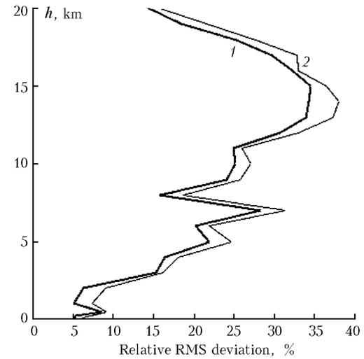
**Fig. 7.** RMS error of retrieval of the vertical profile of water vapor concentration from model spectra neglecting noise (curve 1) and with the ADEOS /IMG noise level (curve 2).
