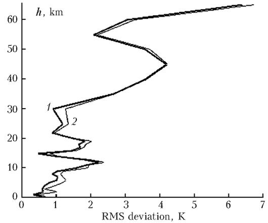
**Fig. 6.** RMS error of retrieval of the vertical temperature profile from model spectra neglecting noise (curve 1) and with the ADEOS /IMG noise level (curve 2).
