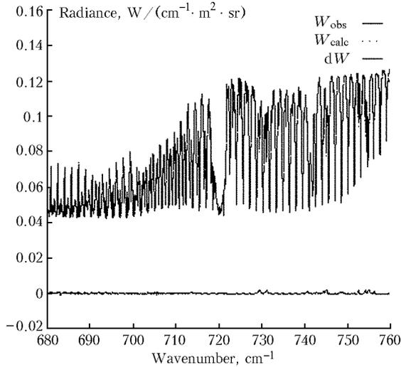
**Fig. 4.** Fitting of the initial model spectrum and spectrum simulated based on the retrieved temperature profile (see Fig. 2).
