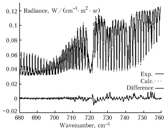
**Fig. 10.** Fitting of the IMG spectrum and spectrum simulated based on the retrieved temperature profile (see Fig. 8).
