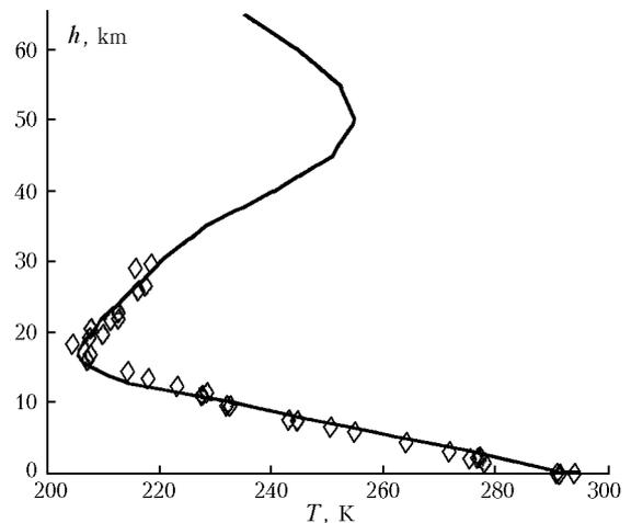
**Fig. 8.** Temperature profile retrieved from IMG spectrum (solid line) along with the radiosonde profile (rhombs) shown for a comparison.
