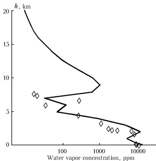
**Fig. 9.** Water vapor concentration profile retrieved from the IMG spectrum (solid line) along with the probe profile (rhombs) shown for comparison.
