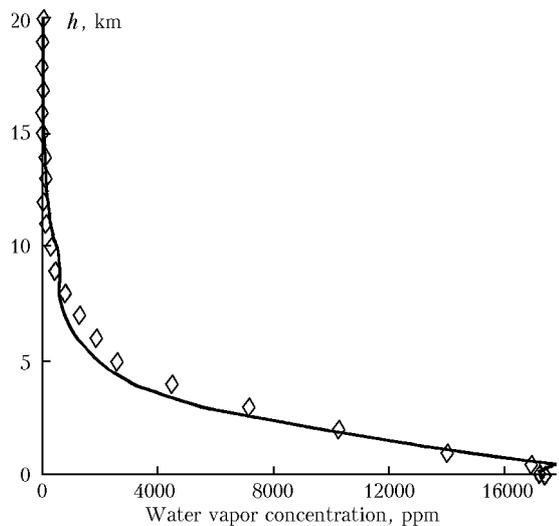
Fig. 3. Initial (solid line) and retrieved (rhombs) vertical profiles of water vapor concentration.
