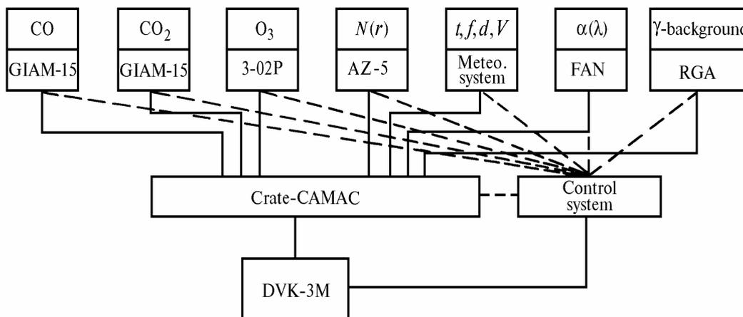
FIG. 1. Schematic diagram of station for atmospheric monitoring (TOR-station).
