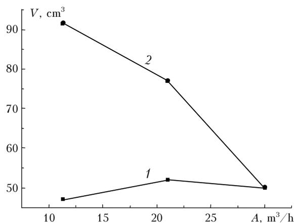
Fig. 3. Gas condensate yield as a function of gas rate.
