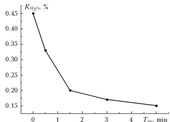
Fig. 2. Variation of water vapor concentration in natural gas as a function of irradiation time at a pressure in the photoreactor of 45 atm.
