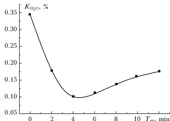
Fig. 1. Variation of water vapor concentration in natural gas as a function of irradiation time at a pressure in the photoreactor of 17.1 atm.
