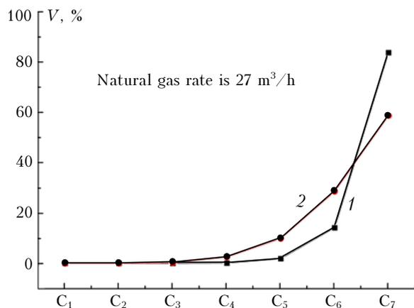
Fig. 4. Content of natural gas before (1) and after (2) irradiation. The pressure at the photoreactor inlet is 45 atm.
