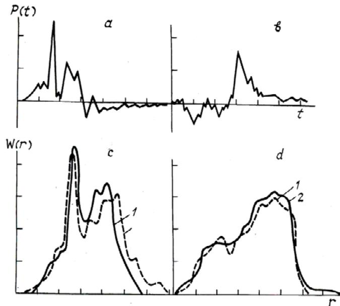
FIG. 2. Acoustic signals recorded at  $T = 12.3^{\circ}\text{C}$ ,  $\rho = 10.5 \text{ g/m}^3$ ,  $c = 0.71$  (a) and at  $T = 0.5^{\circ}\text{C}$ ,  $\rho = 2.8 \text{ g/m}^3$ ,  $c = 1.85$  (b). The  $W(r)$  distributions were retrieved with the help of the above parameters (1) and the bolometric distributions (2). The heat-release time was equal to 0.4 ms (a) and 1.6 ms (b).
