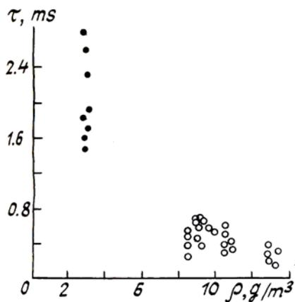
FIG. 3. Heat-release time as a function of the absolute air humidity: points — under KC conditions; circles — without KC.
