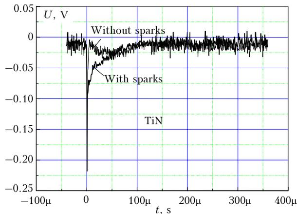
**Fig. 5.** The change of plasma glow (see Fig. 4) intensity with time in the presence and in the absence of sparks.
