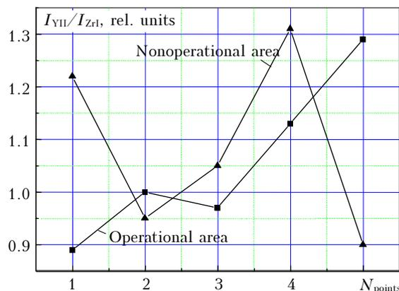
**Fig. 6.** The relation of Y(II) ions radiation intensity at  $\lambda = 4374.9 \text{ \AA}$  to the intensity of Zr atoms glow at  $\lambda = 4710.1 \text{ \AA}$ . The material operational area was used in an installation designed for thin films saturation.
