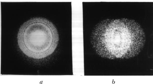
FIG. 3. Interference patterns in the bands of equal thickness recorded when performing spatial filtering in the hologram plane on (a) and off (b) of the optical axis.
