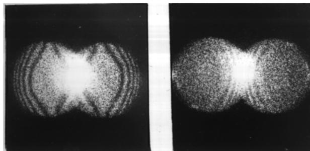
FIG. 6. Lateral shear interferograms in (-1) and (+1) diffraction orders. The amplitude scattering screen is illuminated by a converging, with radius of curvature  $R > l_1$  (a) and diverging with  $R > l_2$ , spherical waves.
