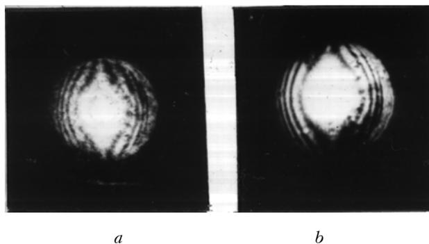
FIG. 5. Lateral shear interferograms localized in the hologram plane reconstructed using a coherent (a) and polychromatic (b) light.
