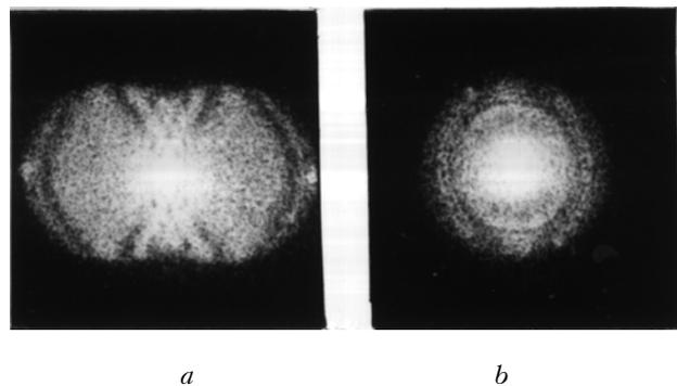
FIG. 4. Interference patterns recorded when performing spatial filtering of the diffraction field in the plane of a double-exposure hologram off (a) and on (b) the optical axis.
