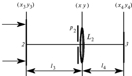
FIG. 2. Optical arrangement of recording interference pattern localized in the hologram plane.
