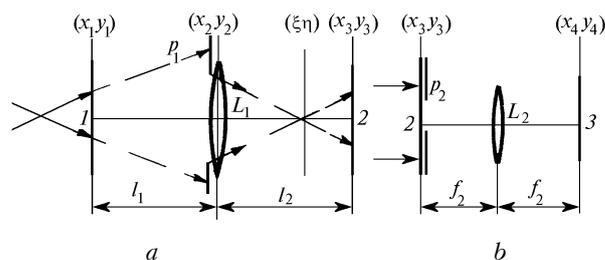
FIG. 1. Optical arrangement of recording (a) and reconstructing (b) of a double-exposure hologram of an amplitude scatterer image: 1, 2, and 3 are amplitude scatterer, photoplate-hologram, plane of interference pattern recording, respectively;  $L_1$ ,  $L_2$  are lenses;  $p_1$  is the objective aperture,  $p_2$  is a spatial filter.
