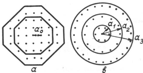
FIG. 2. Diagrams of the positions of the centers of the actuators.
