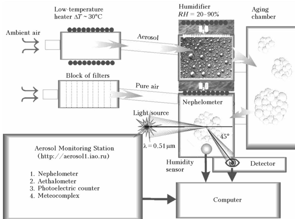
Fig. 1. Block-diagram of the experimental setup.
