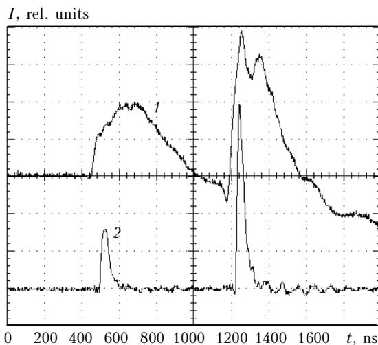
Fig. 1. The oscillograms of current (1) and generation (2) pulses at SrII IR-transitions at  $0.72 \mu\text{s}$  delay between additional and excitation pulses.
