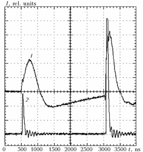
Fig. 2. The oscillograms of current (1) and generation (2) pulses at SrII IR-transitions at  $2.6 \mu\text{s}$  delay between additional and excitation pulses.
