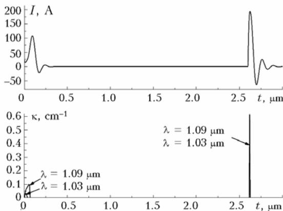
Fig. 4. The calculated additional and excitation current pulses and amplification coefficients at SrII IR-transitions at a  $2.6 \mu\text{s}$  delay.
