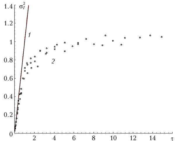
**Fig. 2.** Relative variance of plan wave intensity fluctuations: calculation to the first approximation of MSP (1); simulation (2).
