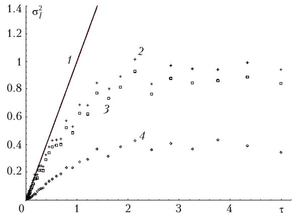
**Fig. 4.** Variance of the received radiation flux fluctuations (plane wave) as a function of optical depth and receiver size to the MSP approximation (1) and at  $a_r = 0.04$  (2),  $0.24$  (3), and  $0.95$  mm (4).
