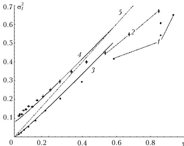
**Fig. 3.** Relative variance of intensity fluctuations of the collimated beam  $a_0 = 3$  cm (the Fresnel number  $\Omega_0 = 57$ ) in the atmosphere with precipitations: rain in the homogeneous atmosphere (simulation and calculation to MSP approximation) (1 and 3); turbulent atmosphere with precipitations, plane wave scintillation index  $\beta_{0,pw}^2 = 0.31C_c^2 k^{7/6} z^{11/6} = 0.1$  (simulation and MSP) (2 and 4); rain in the homogeneous atmosphere, plane wave, MSP (5).
