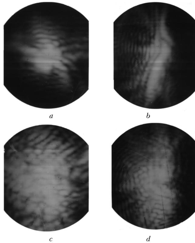
FIG. 3. The photographs of the focal spots of the beam radiation with  $\varnothing = 75$  mm, (a, b) and 150 mm, (c, d) with the thermal heating of the separate area of the optical channel, (b) at the 4 m shortened transportation channel, (c) and the 24 m complete one, (d). The photographs are in about the same scale relative to the diffraction angle.
