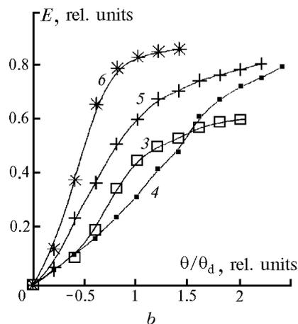
FIG. 2. The angular distribution of the radiation energy, incident on the nonlinear medium (curves 1, 2), (a); the output control laser beam (curve 3), reflected and passed again through the optical channel (curves 4-6), (b); the diameter of the beam is equal to 150 mm (curves 2, 4) and 75 mm (curves 1, 5, and 6); the curve 5 was obtained at heating separate areas of the optical channel.
