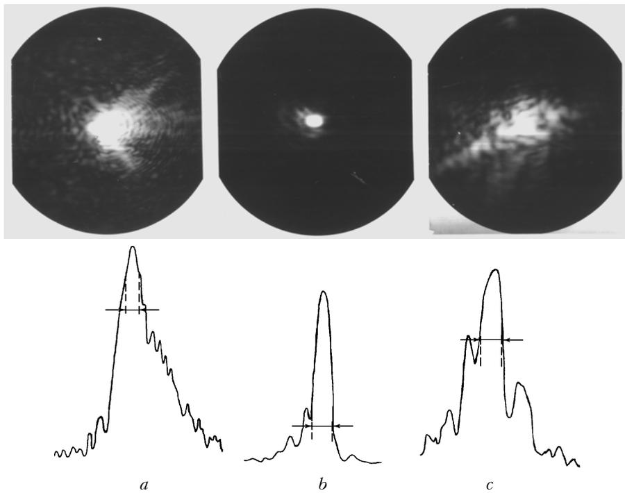
FIG. 4. The photographs of the focal spots and the densitograms of the radiation, reflected from the nonlinear medium and passed again through the optical channel. The diameter of the extended beam is equal to 150 mm, (a) and 75 mm, (b, c). The wave front on the last photographs was distorted additively by the heating of the area of the optical channel.
