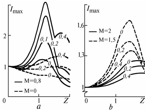
FIG. 3. Variations of maximum intensity in the light beam propagating along the path for different values of the parameter  $\delta$  (adjacent to the curves) in subsonic (a) and supersonic (b) flows of an aerosol medium. Calculation was made for  $N_a = 0$ ,  $N = 1$ , and  $F = 5$ .
