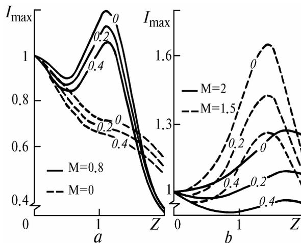
FIG. 2. Variations in the maximum intensity  $I_{\max} = \max_{x, y}[I(x, y)]$  along the path for different values of the aureole scattering parameter  $N_s$  (adjacent to the curves) and light beam in subsonic (a) and supersonic (b) flows of an aerosol medium. Calculation was made neglecting the linear mechanisms of intensity extinction for  $N_a = 0, N = 1, \text{ and } F = 5$ .
