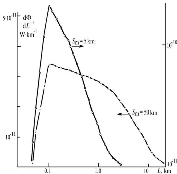
FIG. 3. Differential fluxes of backscattered radiation. Opto-geometrical parameters of lidar visibility meter:  $P_0 = 4.5 \cdot 10^{-2}$  W,  $2\gamma_s = 5'$ ,  $d_s = 0.005$  m,  $2\gamma_r = 22'$ ,  $d_r = 0.1$  m,  $B = 0.2$  m,  $\varphi = 0^\circ$ .
