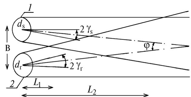
FIG. 1. Geometrical scheme of lidar visibility meter. Source aperture (1) and receiver aperture (2).
