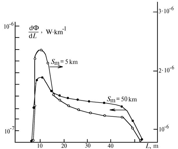
FIG. 4. Differential fluxes of backscattered radiation. Opto-geometrical parameters of lidar visibility meter:  $P_0 = 4.5 \cdot 10^{-2}$  W,  $2\gamma_s = 5'$ ,  $d_s = 0.005$  m,  $2\gamma_r = 1^\circ$ ,  $d_r = 0.16$  m,  $B = 0.25$  m,  $\varphi = 55^\circ$ .
