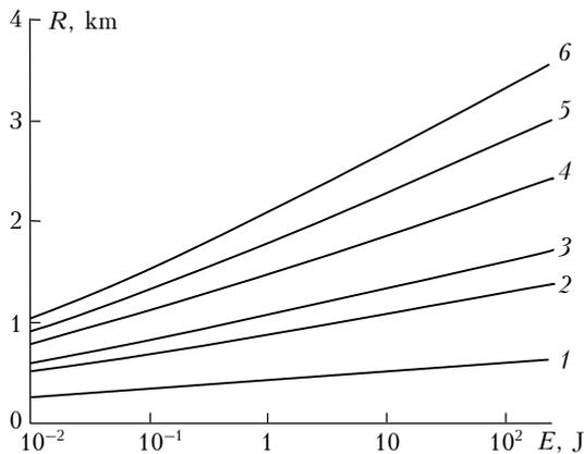
**Fig. 2.** Sensing range as a function of pulse power at  $\epsilon = 1$  for tabun (1), lewisite (2), sarin (3), cyclosarin (4), VX (5), and soman (6).
