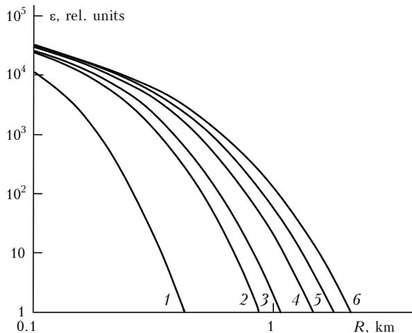
**Fig. 1.** Signal-to-noise ratio as a function of distance for tabun (1), lewisite (2), sarin (3), cyclosarin (4), VX (5), and soman (6) when recording single lidar echosignals.
