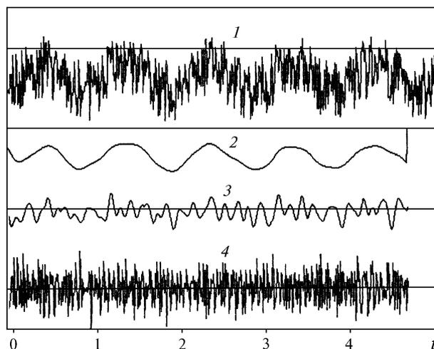
FIG. 2. Versions of the initial signal filtration: the initial curve (1); the result of processing of the initial curve by the low-pass filter with the cut-off frequency of 2 Hz (2); the result of processing of the initial curve by band-pass filter with the transmission frequency of 2–10 Hz (3); the result of processing of the initial curve by the high-pass filter with the cut-off frequency of 10 Hz (4).
