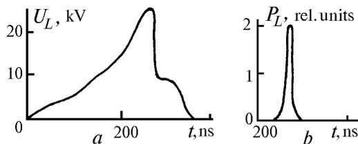
FIG. 7. Waveforms of the voltage at the inductance (a) and laser pulse in nitrogen (b) at  $U_0 = 2$  kV and 30 Torr nitrogen pressure. The crossatron was used as opening switch in this case.
