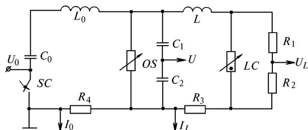
FIG. 1. Circuitry of an inductive storage generator with an opening switch: the opening switch OS, closing switch SC, the laser chamber LC, inductance of the discharge loop with the opening switch and the laser chamber L, voltage dividers  $C_1$ ,  $C_2$  and  $R_1$ ,  $R_2$ , shunts  $R_3$  and  $R_4$ .
