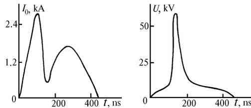
FIG. 2. Waveforms of the total current  $I_0$  and the voltage  $U$  across the opening switch for operation without a load,  $U_0 = 15$  kV.
