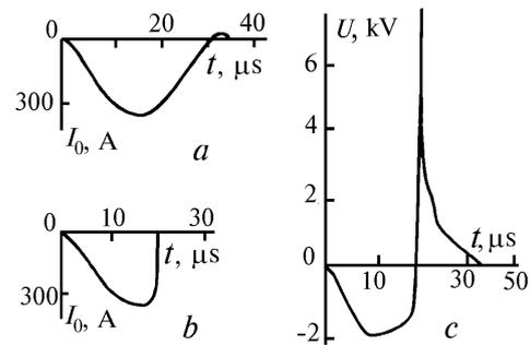
FIG. 3. Waveforms of the total current  $I_0$  without blocking pulse (a), with current interruption (b), and the voltage across the inductance  $L_0$  during interruption (c);  $C_0 = 2$   $\mu$ F,  $L_0 = 32$   $\mu$ H,  $U_0 = 2$  kV.
