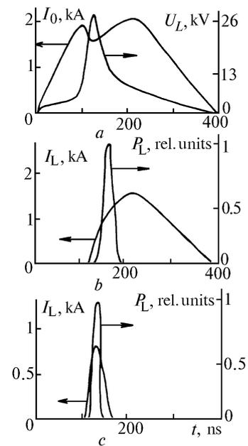
FIG. 5. Time profiles of the total current  $I_0$ , the voltage across the laser gap  $U_L$ (a), the current through the laser gap  $I_L$  and output pulse  $P_L$ (b) under transverse discharge pumping at a nitrogen pressure of 120 Torr and charging voltage  $U_0 = 15$  kV. Waveforms of the current through the laser gap  $I_L$  and laser pulse  $P_L$  under longitudinal discharge pumping at a nitrogen pressure of 15 Torr and  $U_0 = 18$  kV (c).
