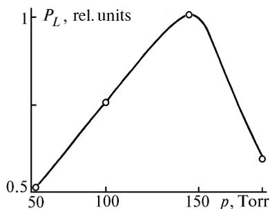
FIG. 6. Output energy as a function of nitrogen pressure under transverse discharge pumping.
