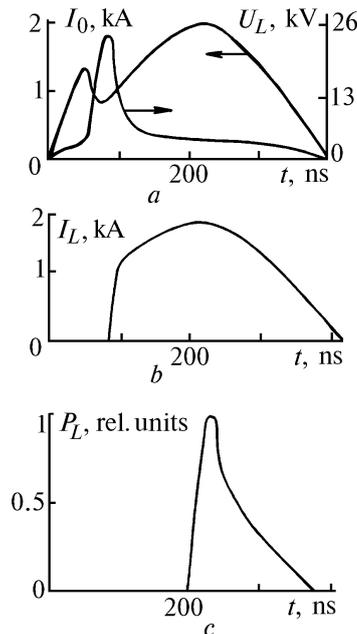
FIG. 10. Waveforms of the total current  $I_0$ , the voltage across the electrodes of the laser chamber  $U_L$  (a), the current through the laser gap  $I_L$  (b) and laser pulse  $P_L$  (c). Gas mixture Ne:Xe:HCl = 160:10:1 at a total pressure of 3.5 atm;  $U_0 = 12$  kV. Electrode separation in the laser chamber was 1.5 cm.
