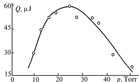
FIG. 9. Output energy as a function of nitrogen pressure at  $U_0 = 20$  kV,  $C_0 = 15$  nF, pulse repetition rate of 2 Hz. Semiconductor opening switch was used.
