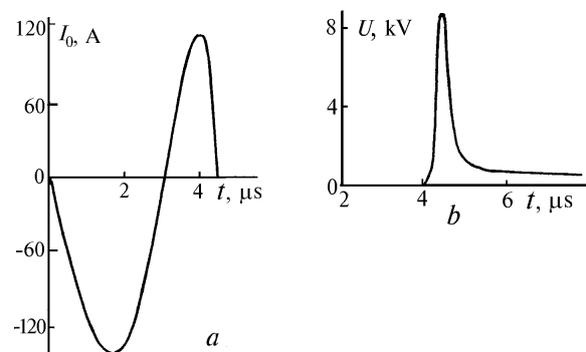
FIG. 4. Waveforms of the current  $I_0$  through the opening switch based on KC-201E diodes and the voltage across the opening switch  $U$  for operation without a load,  $U_0 = 5$  kV.
