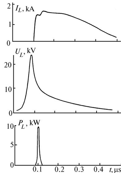
FIG. 8. Waveforms of the discharge current through the laser gap  $I_L$  (a), the voltage across the electrodes of the laser chamber  $U_L$  (b) and laser pulse in nitrogen  $P_L$  (c) at  $U_0 = 20$  kV and nitrogen pressure of 24 Torr. Semiconductor diodes SDL 0.4–800 served as opening switch.
