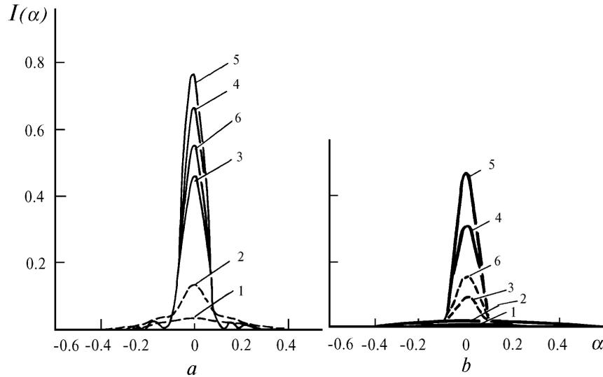
FIG. 1. PSF of an adaptive telescope vs a number of degrees of freedom of an active element: 1) without correction, 2) three degrees of freedom (a segmented mirror and 1 element), 3) 12 degrees of freedom (a segmented mirror and 4 elements), 4) 27 degrees of freedom (a segmented mirror and 9 elements), 5) 48 degrees of freedom (a segmented mirror and 16 elements), 6) 20 degree of freedom (a deformable corrector and 20 servodrives). a)  $r_0 = 20$  cm and b)  $r_0 = 10$  cm.
