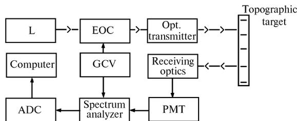
FIG. 2. Schematic of the LFM lidar breadboard construction: laser L, electrooptical converter EOC, and generator of controlling voltage GCV.
