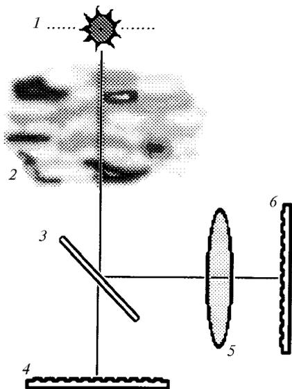
FIG. 1. Diagram showing the experimental configuration of optical system considered in the numerical experiment: 1) plane of a light source, 2) turbulent medium, 3) light-splitting plate, conjugation plane, 4) and 6) receivers, and 5) Fourier transformer.
