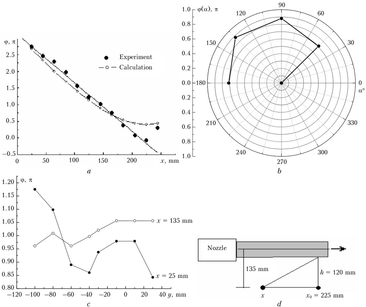
**Fig. 4.** The phase shift of acoustic waves in measurements by configurations of Fig. 1a (a); Fig. 1b (b); Fig. 1c (c) and the illustration to the calculation of phase shift (d).
