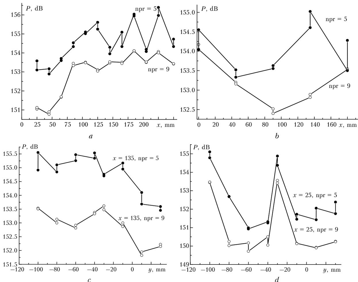
**Fig. 6.** The level of acoustic oscillations at  $npr = 5$  and  $9$  with configurations: along the axis (*a*), in a circle (*b*), in the transversal section at  $x = 135$  mm (*c*) and  $x = 25$  mm (*d*).
