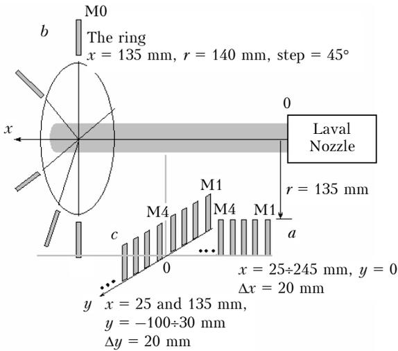
Fig. 1. Configurations of microphones in the Eifel chamber.
