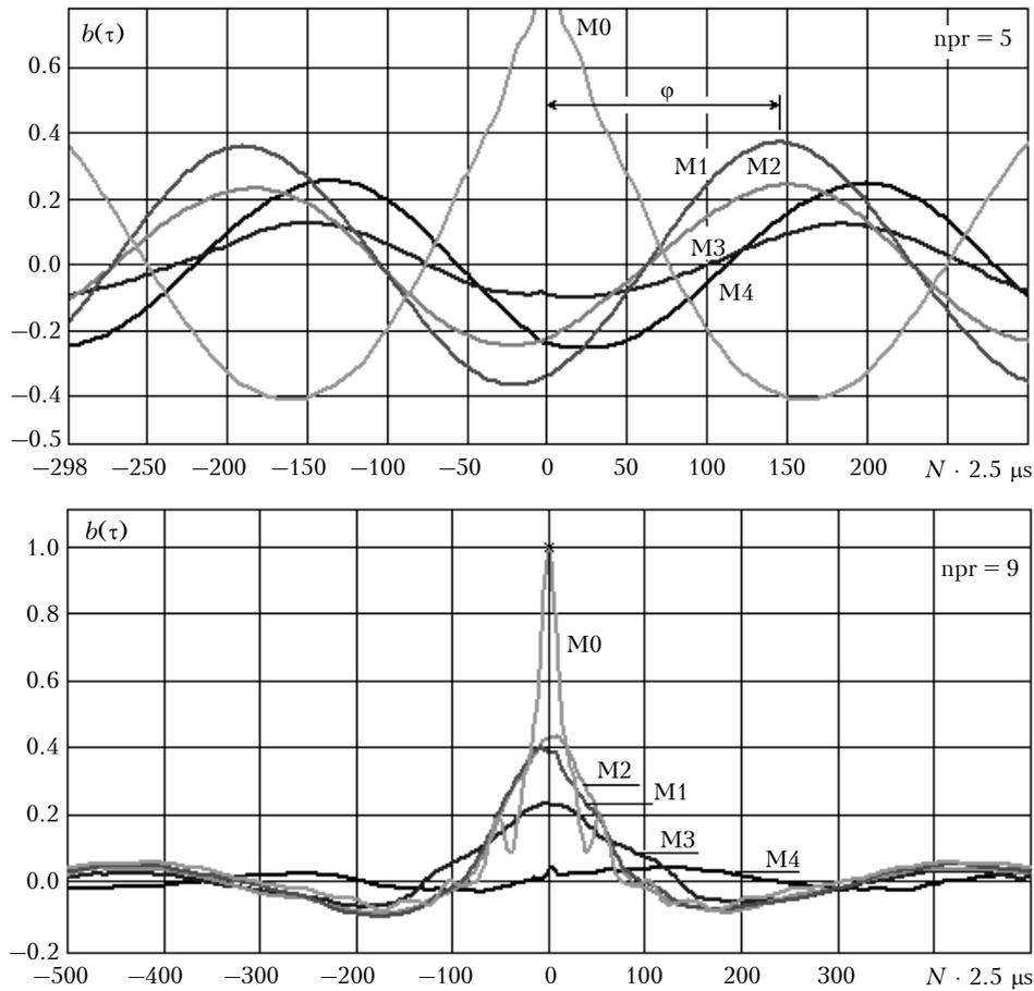
**Fig. 3.** Coefficients of time correlation of acoustic wave. M0 is the coefficient of autocorrelation of the first microphone, M1... M4 are the coefficients of cross-correlation between the microphone M0 and microphones M1, M2, M3, M4;  $\varphi$  is the phase shift.
