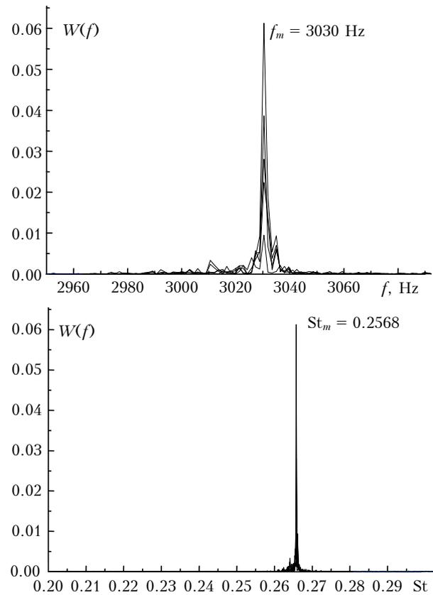
Fig. 2. Spectra of acoustic wave fluctuations at  $npr = 5$ .
