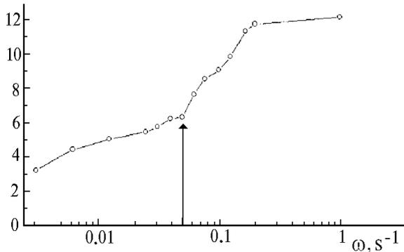
FIG. 2. Spectrum of the estimate from above of the LF component of the PSF signal shown in Fig. 1. The cutoff frequency is indicated by the arrow.
