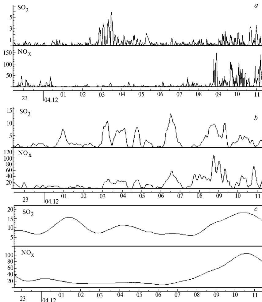
FIG. 4. Result of frequency selection of the data presented in Fig. 3 by the PSF method: a) high-frequency component; b) middle-frequency component; c) low-frequency component. Characteristic times are 5 and 60 min. Concentrations are in ppb.
