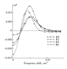
FIG. 1. SPectral dePendences of differences between the monochromatic transmission functions for Voigt and Galatry lineshaPes for different HCl lines at the sighting height  $h_0 = 20$  km.
