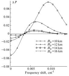
FIG. 2. SPectral dePendences of the differences between the monochromatic transmission functions for the Voigt and Galatry lineshaPes of the H<sub>2</sub>O line at different sighting heights ( $v_0 = 3950.271 \text{ cm}^{-1}$ ).
